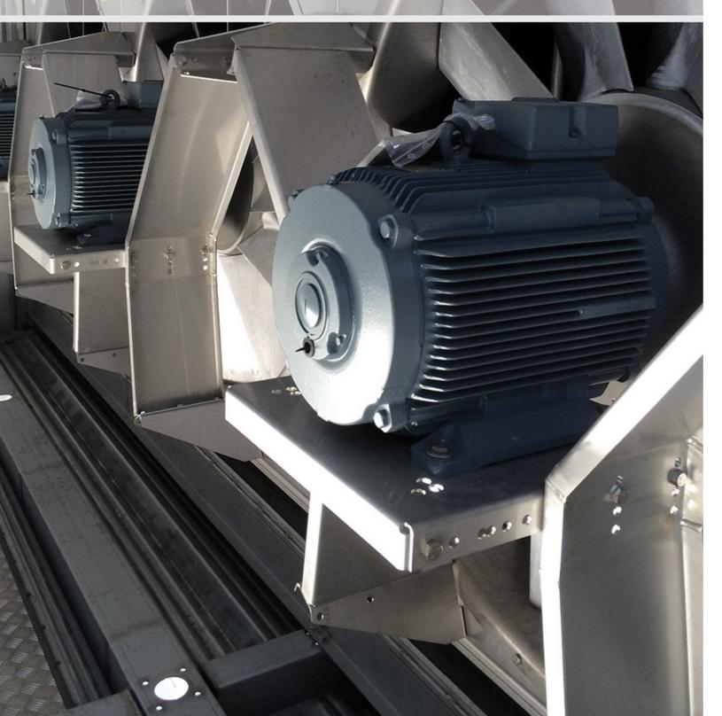
The motor in the drying process circulates air and heat. The circulating air in the dryer has several tasks. When air blows through the heating coils, it gets heated up. When the heated air blows through the timber stacks, it is transmitting energy to the timber, which is beeing used for evaporation of water. The air also removes the evaporated water from the wood surface. The energy beeing used for evaporation of water comes with a price.
