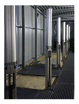
climates well over Plasticity Level and at same time adding pressure on top of the stacks during entire Process, we are causing permanent deformation in cell structure, giving you straight and stress free timber, happy Customers and higher Margin as final result.
