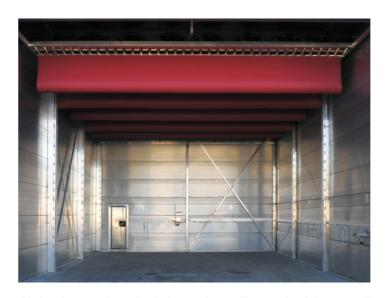
Air baffles are installed above the ceiling of the kiln as well as in the side walls to prevent the leakage of airflow outside of the timber stacks. They ensure a reinforcement of air circulation through the timber stacks and maximise the active airflow process in the stacks. Their installation leads to an improvement in the quality of the drying while reducing power consumption. Air baffles come in various
