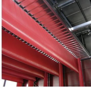
materials and mechanical models. The final recommended combination is offered according the specific conditions of each client. Air baffles are a very important part of our kilns and have a significant impact on the final quality of the dried material and economy of the entire drying process.
